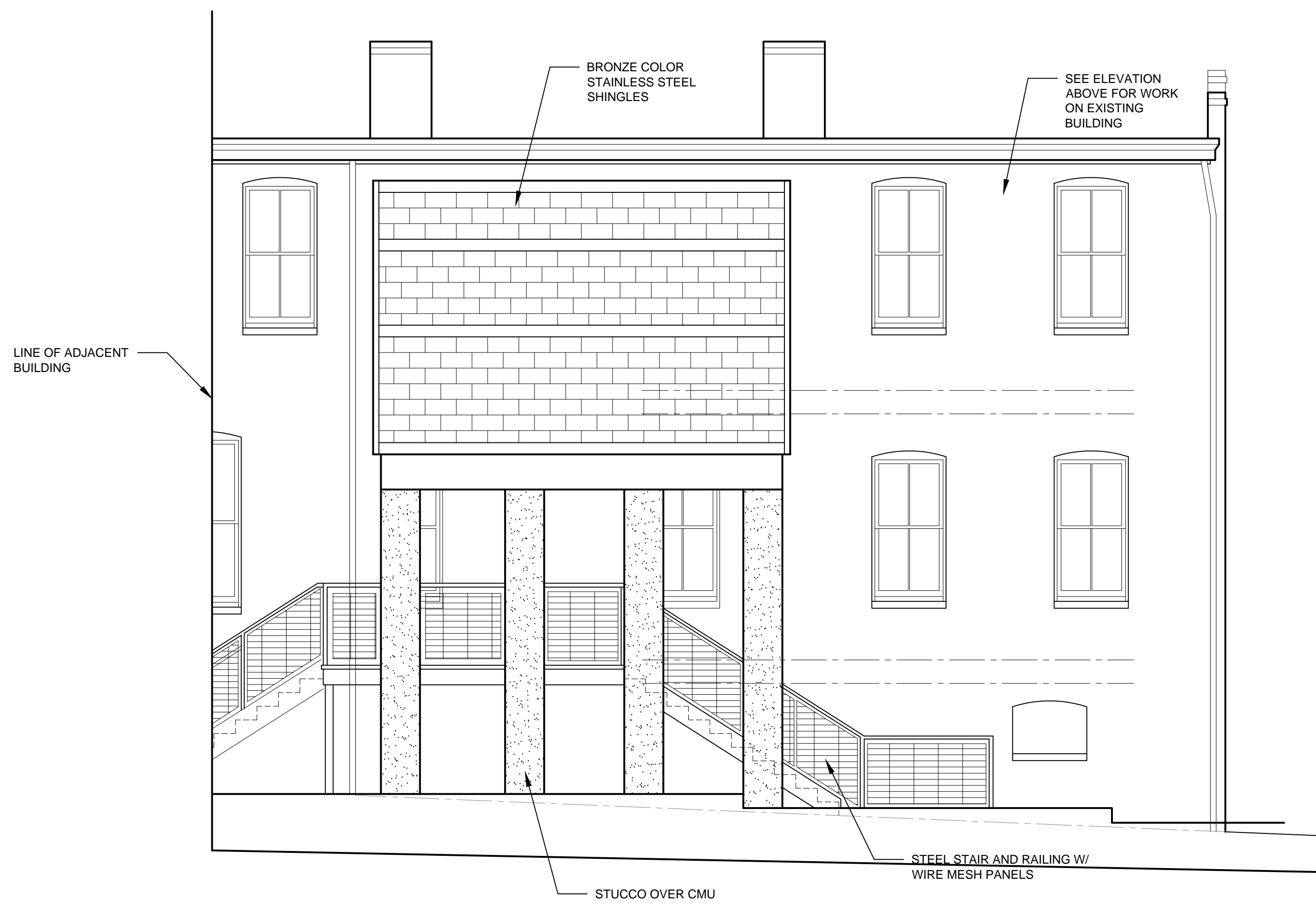
WEST SDE ELEVATION - WITH ADDITION
